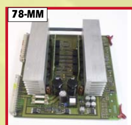
78-MM LTK-500 Later Version Power Port Board 500w #91.144.8062
