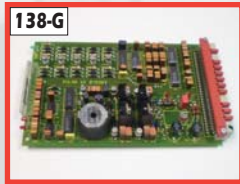
138-G KK #PO.016263 Monitoring Channel Card
