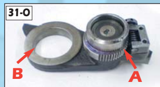
31-O Operator Side Upper A Block for Bearing #66.030.007 B Swiveling Lever #93.030.005
