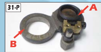
31-P Operator Side Lower A Block for Bearing #93.030.011 B Swiveling Lever #93.03.004
